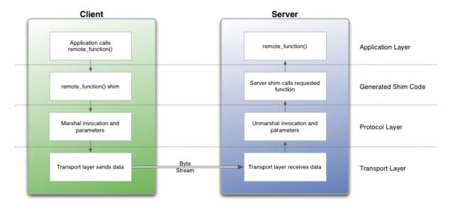
RPC implementations typically use a combination of a tool (erpcgen) and IDL (interface definition language) file to generate source code to handle the details of marshaling a function's parameters and building the data stream.
