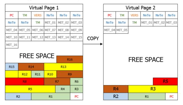
Finally, the virtual page 2 is validated by writing the PC value and a request to erase virtual page 1 is performed. The page is erased on an idle task, sector by sector where only one sector is erased at a time when idle task is executed.
