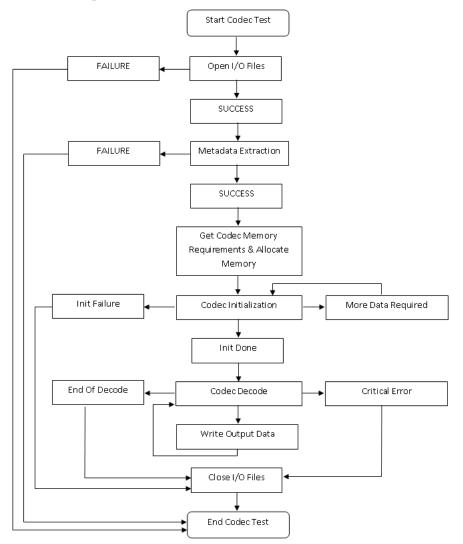
Adding new decoders to the CCI This section explains how to integrate a new decoder in the Common Codec Interface. The CCI assumes the decoder library to be used is in the  $\middleware\audio\_voice\audiocomponents\decoders\*decoder*\libs\ folder of the maestro framework. The CCI is just a wrapper around a specific implementation. The decoder is expected to be extended as needed to meet the APIs described above.$
