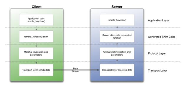
RPC implementations typically use a combination of a tool (erpcgen) and IDL (interface definition language) file to generate source code to handle the details of marshaling a function's parameters and building the data stream.
