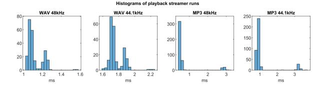
**Time on each element** In the tables and histograms below, the timings for individual elements and their connections are provided. Given that the file reading function was invoked during the codec's operation, the tables for individual elements display the total time on the codec element, the time on the codec element before the file read, and the time on the codec element after the file read. The individual blocks in the tables are as follows:
