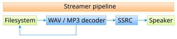
The measurement of streamer pipeline run started at the beginning of streamer\_process\_pipelines(): streamer.c and ended in the function streamer\_pcm\_write(): streamer\_pcm.c just before the output buffer.
